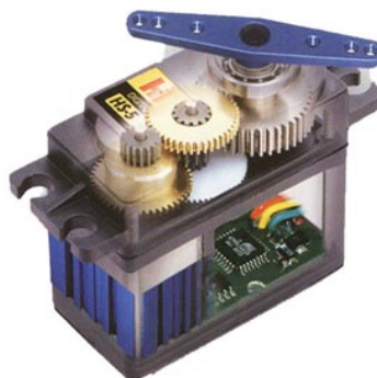
Figure 5.1: Servo internals. Source: hitecrcd.com
